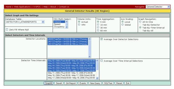
FIGURE 3 The V-SPOC General Detector Results screen. The purpose of this screen is to refine the detector database query parameters with respect to detector and time interval selections, detector variables (volume, speed, and occupancy), aggregation levels, and presentation attributes.
