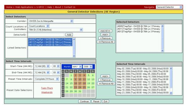
FIGURE 2 The V-SPOC General Detector Selections screen. The purpose of this page is to fix the spatial (list of detectors) and temporal (list of time intervals) dimensions for the resulting detector database query.
