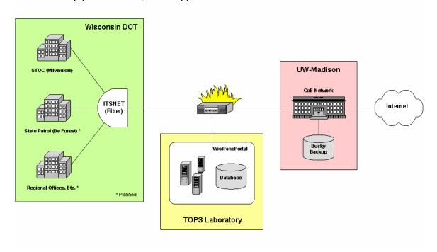
FIGURE 1 High level overview of the WisTransPortal network architecture. The WisTransPortal sits directly on the UW College of Engineering network and connects to WisDOT over the ITSNET fiber backbone or via the internet.
